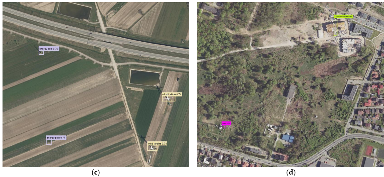
Figure 11. Sample detection (fragment of orthophotomap): (a) construction cranes; (b) wind turbines and energy poles; (c) wind turbines and energy poles; (d) construction crane and mast.
